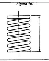
VALVE SPRING FREE LENGTH GN190: 1.910 inch (48.48mm) GN220: 2.074 inch (52.69mm)
